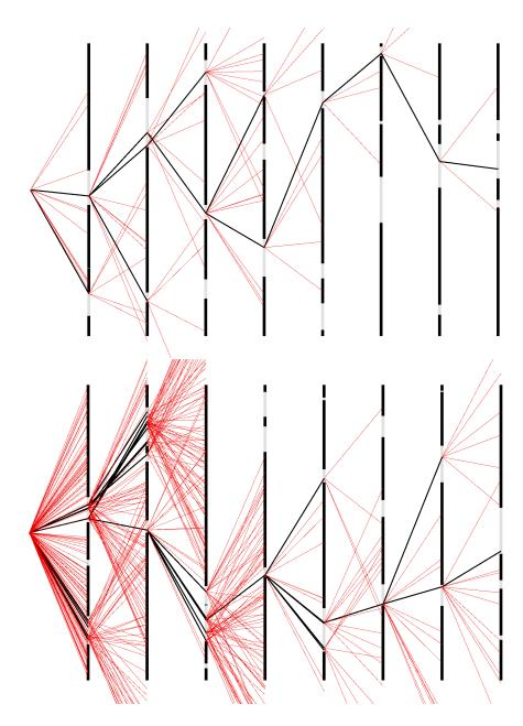
Figure 5.2: An example of a randomly generated world with 8 gates. The black regions are barriers. The planner starts at the left, and it samples configurations until it reaches the right. The top diagram shows paths found using the MCTS strategy, and the bottom shows paths found using the normalized strategy. Red paths are failures while black paths were successful.
