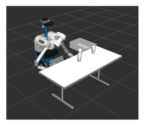
Figure 6.2: The task used for comparing strategies for interleaving planning and execution. The robot must move all three glasses into the bin.
