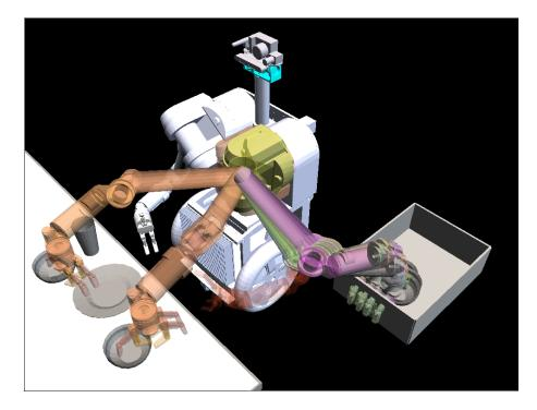
Figure 1.2: A visualization of some intermediate states for a path through configuration space that moves all items from a table to a bin.
