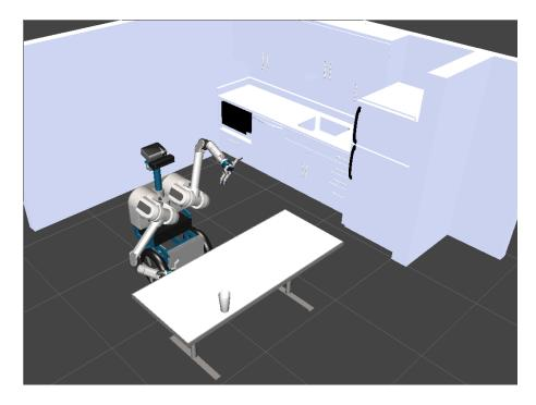
Figure 1.1: An example of a long horizon manipulation task. The robot must move the glass from the table to the kitchen counter.
