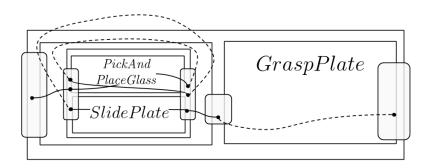
Figure 4.2: A graphical representation of the table reconfiguration task. Dashed lines signify configurations that are shared. In this case, configurations that did not make it into the goal set are returned to the start set of the repetition action. This happens twice, corresponding to two glasses that had to be moved before the plate could be slid.
