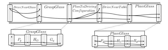
Figure 4.1: The task specification for a pick and place task that includes base movement.
