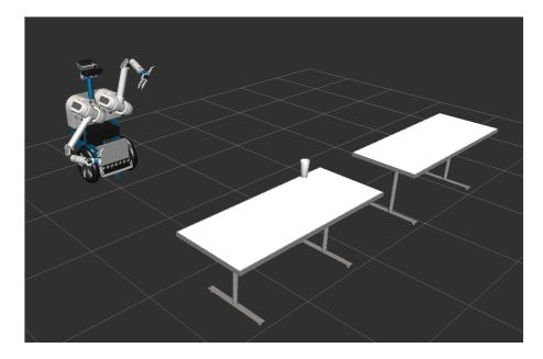
Figure 5.5: The Pick and Place Task. The robot must move the glass from one table to the other.
