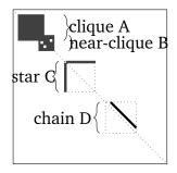
Figure 3.2: Illustration of our main idea on a toy adjacency matrix: VoG identifies *overlapping* sets of nodes, that form vocabulary subgraphs (cliques, stars, chains, etc). VoG allows for the soft clustering of nodes, as in clique A and near-clique B. Stars look like inverted L shapes (e.g., star C). Chains look like lines parallel to the main diagonal (e.g., chain D).
