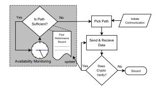
Figure 1: High-level control flow diagram of ACR.
