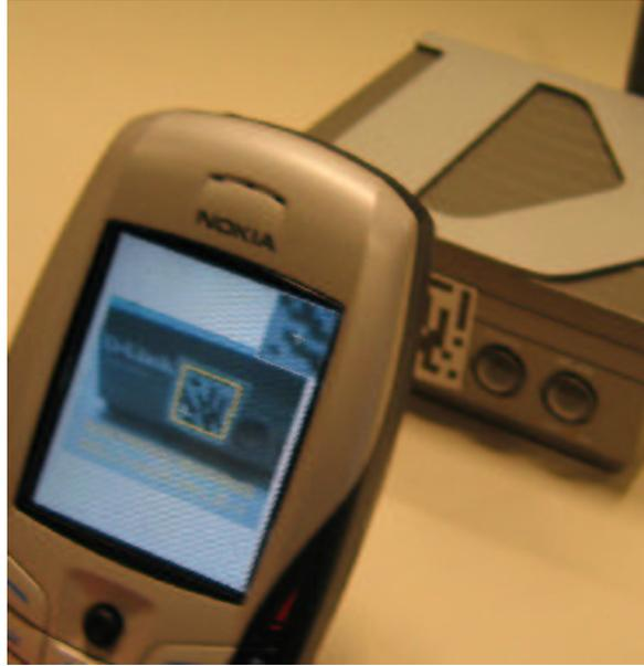
Figure 3: Phone running SiB scanning a barcode on an 802.11 wireless base station.
