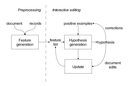
Figure 9.15: Block diagram of simultaneous editing algorithm.
