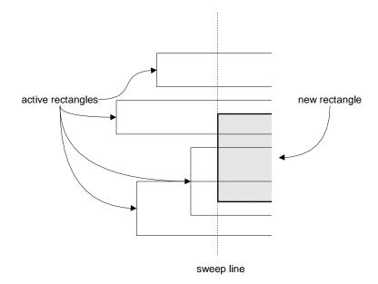
Figure 4.16: The plane-sweep intersection algorithm (after Preparata & Shamos [PS85], Figure 8.29).
