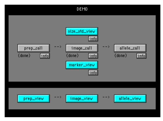
**Figure 8.6.** Dependency chart of FAST-MAP programs for another scenario. The top pane lays out the *obligatory* programs to call, with the program dependencies displayed from left to right, and top to bottom. The bottom pane shows the optional viewing programs at the various programmatic checkpoints for the user to verify and correct intermediate results.
