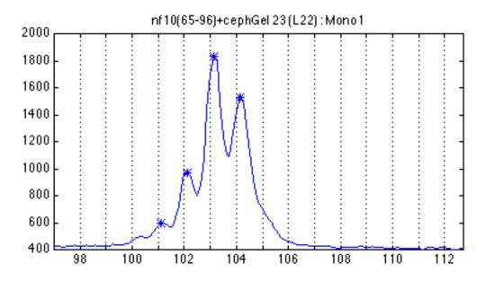
**Figure 9.8.** An electropherogram trace for Mono1, a TET-labeled mononucleotide marker with the size range of 100 to 110 bp. Shown here is a heterozygote which has alleles that are separated by only 1 bp (103 bp and 104 bp).
