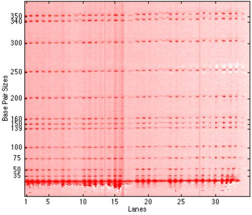
**Figure 4.7a.** The gel image for the TAMRA dye after the application of the refined dye matrix  $D_{refined}$  on the raw data. See also the gel image shown in Figure 4.2a for comparison.
