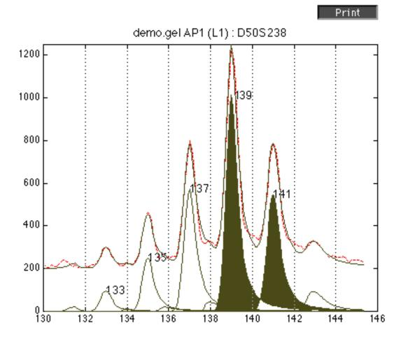
**Figure 8.14.** The expanded view from the quantitation display pane of the main *allele\_view* window. This window shows original electropherogram (dashed line) overlaid with the computed fit (solid line) for comparison. The individual fitted peaks are shown below the electropherogram, and they are labeled with the respective binned alleles. The two bands that correspond to the called alleles are shaded.
