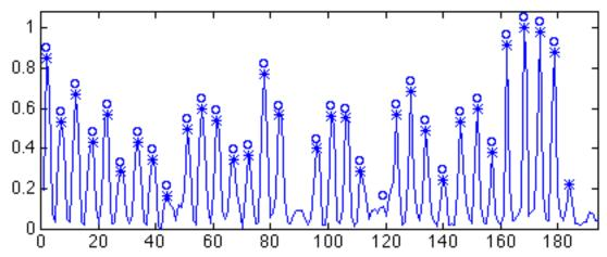
**Figure 4.8a.** The projection profile of the best horizontal subsection in the gel. The locally detected data peaks are marked "\*", while the "o" markers indicate the final mapped lane locations using the gel's expectation layout information.
