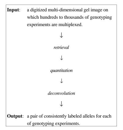
**Box 3.1.** The overall data flow in the genotyping problem. The input data is a highly multiplexed gel image, from which we retrieve the data window for each multiplexed experiment for analysis, quantitate the extracted signal data into molecular units, and deconvolve the complex data patterns to accurately call the two alleles in the genotype.
