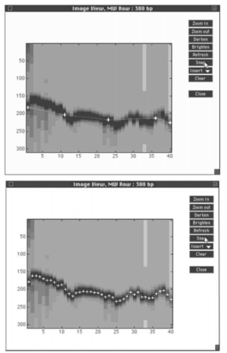
**Figure 9.1.** Custom "snap-to" ImageView ALF interface. Top: The user clicks on several size standards to suggest where the size standards are. Bottom: The computer automatically fills in the rest of the size row, and then calibrates the DNA sizes in every lane.
