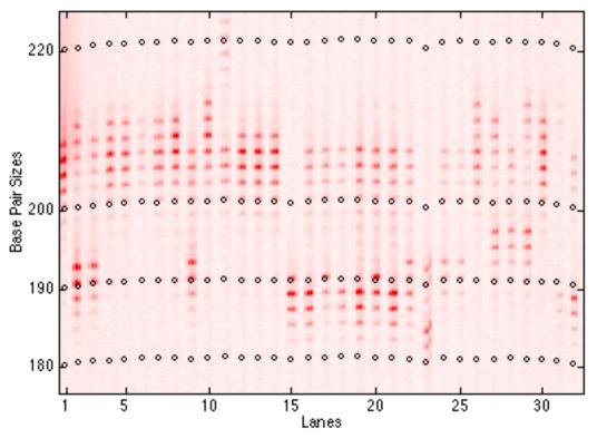
**Figure 5.4.** The marker image for the TET-labeled dinucleotide D16S511. There are 32 lanes on the gel shown. The "o"s indicate the locations of the MW (Bioventures 20 bp ladder) sizing grid from the TAM dye plane. The highest resolution provided is 10 bp,
