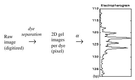
**Figure 3.1.** Retrieving data from gel. First, the raw digitized image from the DNA sequencer is separated into two-dimensional gel images for each fluorescent dye used in the experiment. Then, the coordinate transformation function  $\alpha$  converts the gel image into linear electropherogram traces of microsatellite data in each lane, calibrated by DNA size instead of pixel.
