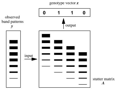
**Figure 6.5.** The GMBD procedure. The stutter matrix *A* is divided by the observed (input) data vector *y* to compute a best-fit (output) genotype vector *x*.
