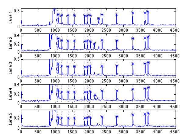
**Figure 4.9c.** The detected ("\*"'s) and mapped (dashed lines) MW bands for the first 5 lanes of the gel. Notice how the bleedthrough bands have been avoided by the expectation-based approach.
