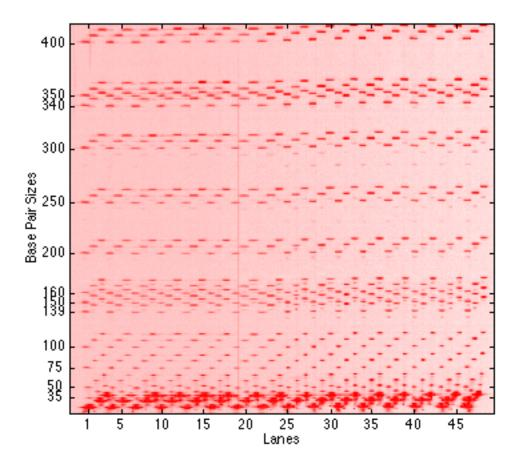
**Figure 4.4b.** Another example of staggered loading. On this 48-lane gels, sets of lanes were loaded at three different times. First, lanes 1, 4, 7, and so on were loaded. Then, lanes 2, 5, 8, and so on were loaded. Finally, the remaining lanes, lanes 3, 6, 9, and so on, were loaded. This resulted in a complex zig-zagging pattern that is very different from the one shown in Figure 4.3a. (*Provided by Frosti Palsson, deCODE Genetics, Inc., Inceland.*)
