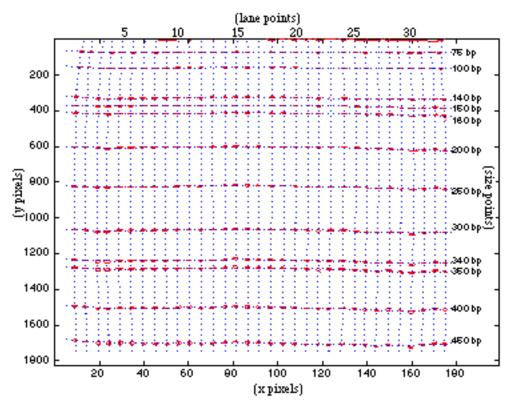
**Figure 3.2.** A sizing grid constructed from the MW size standards data. The vertical grid lines are the lane traces; the horizontal grid lines are contour lines of identical MW mobility and size. The sizing grid is useful for localizing expected marker allele events on the gel image.
