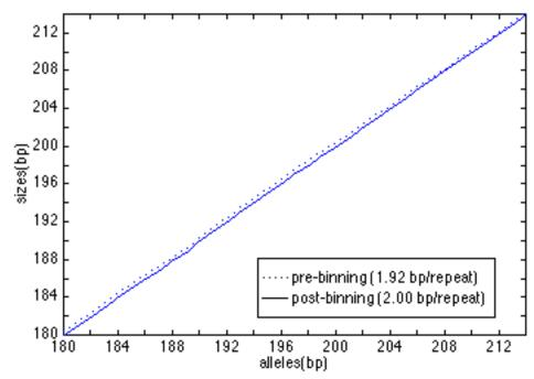
**Figure 5.7.** The size calibration curves for the dinucleotide D16S511. We plot the interpolated sizes against the actual allele sizes. With the MW-sizing grid ("pre-binning"), the slope gives 1.92 bp/repeat, whereas with the marker-adjusted grid ("post-binning), the sizing slope is an accurate 2.00 bp/repeat.
