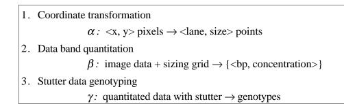
**Box 3.2.** Data transformations in solving the genotyping problem: (1) image pixel coordinates are transformed to facilitate data extraction, (2) data bands are quantitated into molecular units, and (3) stutter data tare deconvolved into recover the true alleles in the genotypes.
