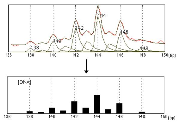
**Figure 5.15.** Band quantitation output. The top pane shows the final sum of fit (solid line) and the individual peaks beneath it. The bottom pane shows the output of the band quantitation step: each darkened bar represents a discretized data band located at an integral allele size. The heights of the bars depict the computed relative DNA concentrations.
