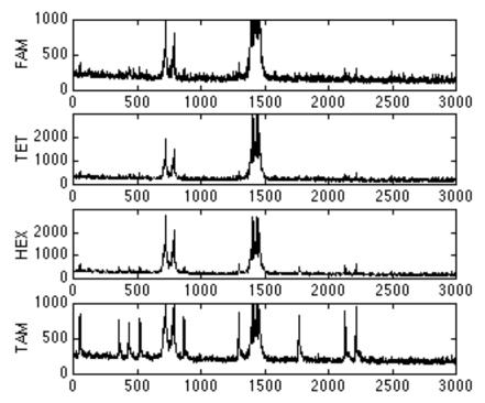
**Figure 4.6a.** The signal intensity profiles from the raw data from the laser sensors for each of the fluorescent dyes. Without applying the dye separation matrix, there is a high degree of dye bleedthrough. For example, the data signals between scan columns (x-axis) 500 and 1000, as well as those near scan column 1500, showed up in the intensity profiles of all the dyes.
