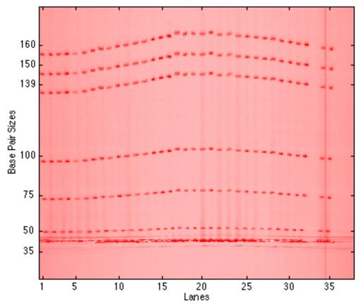
**Figure 4.3a.** Gel smiles. Instead of forming *straight* rows across the lanes, the identical sizing DNA fragments loaded in each of the 34 lanes on this gel migrated at different rates in different lanes, resulting in curved rows ("smiles") across the lanes. (*Provided by Dr. Charles Mein, University of Oxford.*)
