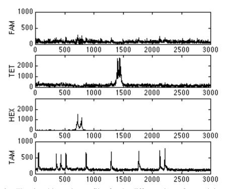
**Figure 4.6c.** The signal intensity profiles for the different dyes after applying the corrected dye separation matrix  $D_{refined}$ . The data bands from dye HEX no longer bled into the dye images for TAM and FAM, and the bleedthrough bands from the TET dye have also been eliminated from the data for the HEX dye.
