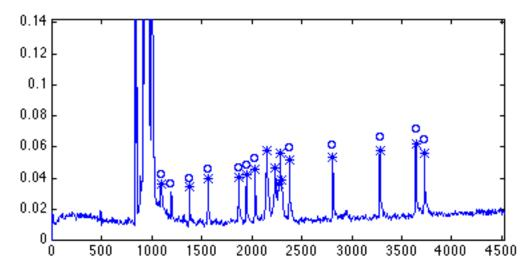
**Figure 4.9b.** An example in which the bleedthrough bands (in the middle region) are of higher signal intensities than the actual MW bands.
