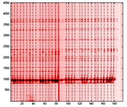
**Figure 4.8c.** The piece-wise constant lane template (dashed lines) constructed from the lane locations from the various cross sections on the gel. Only the tracks for the 32 loaded lanes are shown over the gel image.
