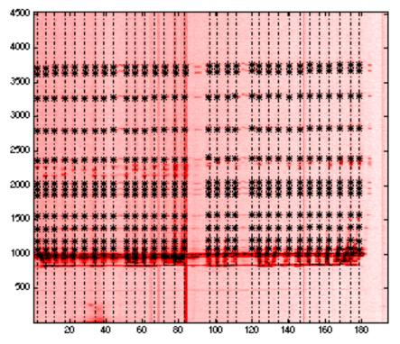
**Figure 4.9d.** MW calibration of the 32 loaded lanes. The dashed lines show the piece-wise constant lane templates constructed by TRACK\_LANE. The "\*"'s mark the mapped MW bands in each of the loaded lanes by CALIBRATE\_MW.
