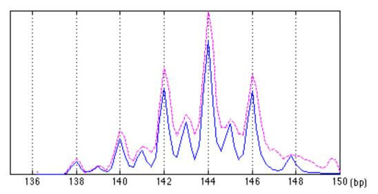
**Figure 5.10.** Initial sum of fit. The solid line shows the initial sum of the fit from iteratively estimating an initial fit for each detected peaks individually. The original electropherogram is plotted with a dashed line (of a lighter color) above the fitted profile.
