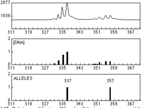
**Figure 6.15.** Relative amplification. When the alleles in a genotype are widely separated (with respect to their sizes), they may not be amplified in an 1:1 ratio. Here, the bands for the bigger allele (357 bp) are considerably less amplified than the bands for the smaller allele (337 bp).
