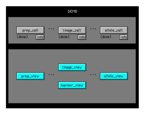
**Figure 8.5.** Dependency chart of the programs to call in FAST-MAP. If the data is relatively perfect and there is no need for the user to verify intermediate results, then one needs only run *allele\_call*. Otherwise, the user may elect to call intermediate programs (in the top pane), and optionally use the viewing programs (in the bottom pane) to check the intermediate results before proceeding further.
