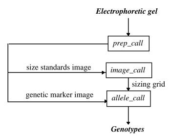
**Figure 8.3.** Data flow between FAST-MAP's core programs. The core programs consist of: *prep\_call*, which prepares sequencer-specific gel data for FAST-MAP by extracting gel images from the raw data, *image\_call*, which constructs the sizing grid, and *allele\_call*, which calls the alleles for every genotyping experiment on the gel.
