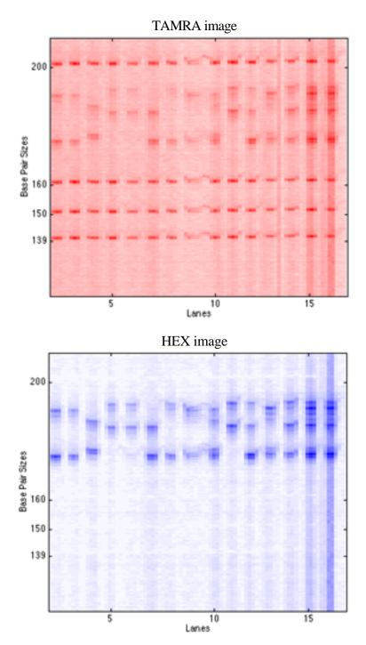
**Figure 4.2b.** We zoom in to the gel region between 160-200 bp, and lanes 1 through 15 for the gel shown in Figure 4.2a. On the top is the gel image for the TAMRA dye, below it is the image for the HEX dye for the same gel region. The data bands from the marker in the HEX dye have clearly bled into the TAMRA dye image.
