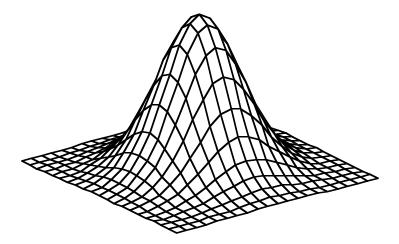
**Figure 9.14.** A 3-D Gaussian model for gridded filter spotting. Using this mathematical model to fit the filter spots, we can systematically eliminate diffusion effects, and quantitate the spots by computing the volume under the curve.
