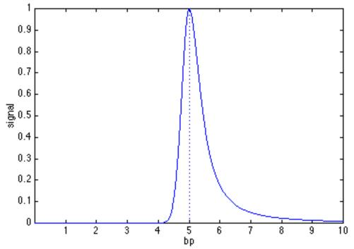
**Figure 5.8.** Gauss-Runga model function. The center of this peak is at the 5 bp mark. Its Gaussian half width for the left half is 0.33 bp, and its Runga scale is 2.17 for the trailing right half.
