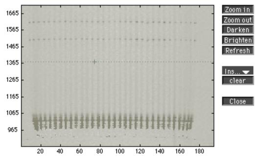
**Figure 8.8.** Cropping away primer region in *prep\_view*. To crop the primer region away from the gel, the user click at one or more minimum scan locations (shown here as a "+"). The computer automatically extends the clicks into a minimum scan line (shown as a horizontal dotted line) separating the primer region from the data.
