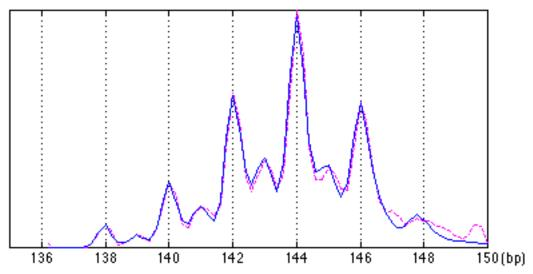
**Figure 5.13.** Sum of fit (dark solid line) after locally optimizing the peak heights (*h*) of each detected marker peaks. This is a fairly close fit to the original electropherogram (light dashed line) after one round of locally optimizing peak parameters.
