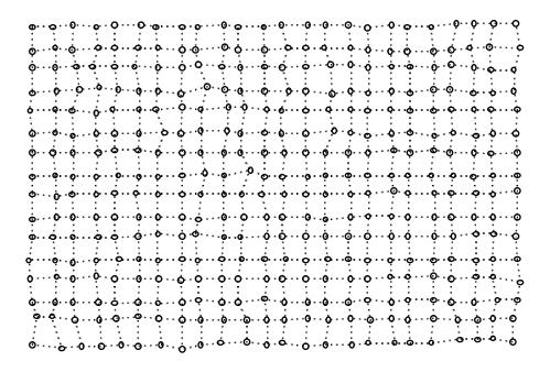
**Figure 9.13.** A spotting grid for the gridded filter shown in Figure 9.12. The grid was constructed automatically based on robotic gridding information. With this grid, the computer can localize the 384 gridded spots on the image, and focus its computation on the 384 local subproblems.
