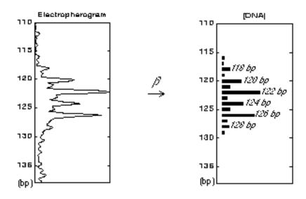
**Figure 5.1.** Band quantitation. This involves converting the continuous electrophoretic signals (shown on the left) into discrete data bands (shown on the right), assigning an integral size to each of the data bands detected, and determining the relative DNA concentrations of the data bands.
