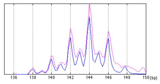
**Figure 5.11.** Sum of fit after locally optimizing the Gaussian half-widths ( $\sigma$ ) of the detected marker peaks. The resulting sum of fit (dark solid line) shows noticeably closer fit to the original electropherogram (light dashed line) on the left sides of the marker peaks. This is because under our peak model, only the left halves are Gaussian.
