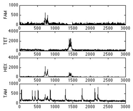
**Figure 4.6b.** After applying the dye separation matrix  $D_{given}$ , it became clear that the data bands between scan columns 500 and 1000 belonged to the HEX dye, whereas the bands around scan column 1500 belonged to the TET dye. However, the bleedthroughs have not been totally eliminated. For example, some of the data bands from the HEX dye can still be found in the data for the TAMRA (labeled as TAM here) and FAM dyes, and some of the bands from the TET dye.
