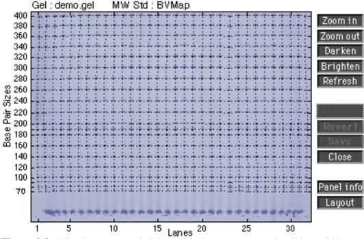
**Figure 8.9.** Viewing computed sizing grid. In *image\_view*, the sizing grid is overlaid on the gel image, allowing the user to verify the correctness of the grid at one glance.
