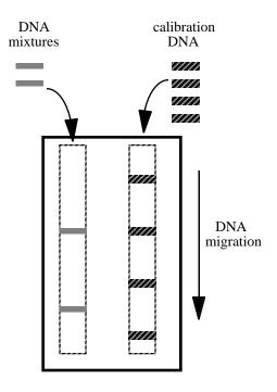
**Figure 2.6.** Gel electrophoresis. DNA of different sizes migrate at different speeds in a gel subjected to an electric field. Typically, calibration DNAs with known sizes (molecular weight standards) are run together with the unknown DNAs so that the unknown DNAs can be typed by size interpolation.
