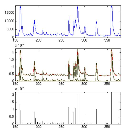
**Figure 9.11.** A FAST-MAP viewing window adapted for displaying quantitative DD analysis. Pane 1 shows the electropherogram trace, pane 2 the quantitative fit of model peaks to data, and pane 3 the final quantitation results.
