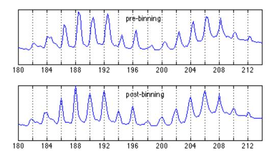
**Figure 5.6.** Sizing grid refinement. In the top pane, the pre-binning MW sizing grid is overlaid on the superimposed electropherogram of 32 lanes of D16S511 (see also Figure 5.3). The marker bands lie slightly off the MW sizing grid. In the bottom pane, the post-stutter crawling grid is overlaid. The marker bands now snap tightly to the refined grid.
