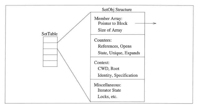
The setObj structure is the basic data structure for a set. It contains an array of per-member data, counters, some of the state of the creating process, iterator state, and a lock to provide mutually exclusive access to the set.
