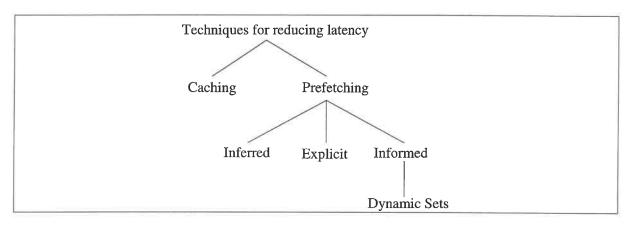
This figure shows the hierarchy of techniques to reduce latency. The dynamic sets abstraction is an example of informed prefetching. The other techniques are either not effective for search, or complicate the programming model.
