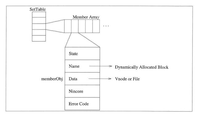
The memberObj structure holds information on one member of a set. This information includes the member's name, a pointer to its data, an error code, and two counters.
