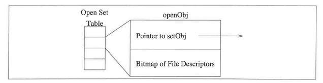
The openObj structure contains the per-process state of a set. This consists of a reference to the setObj and an indication of which of this process's open files belong to (are members of) this set.
